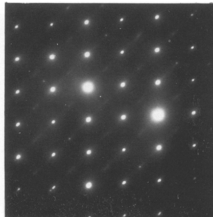
Figure 5 Transmission electron micrograph of a zirconium titanate pocket contained within a tetragonal zirconia grain. B_{\text{Titanate}} = [121] .
