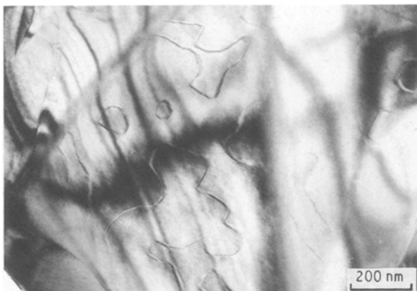
Figure 17 Transmission electron micrograph of an area of monoclinic phase containing APBs. Imaged under multibeam conditions.
