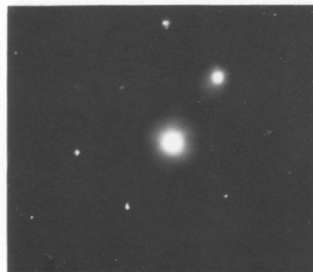
Figure 12 Transmission electron micrograph of an isolated pure TiO_2 particle. B is close to [011] .
